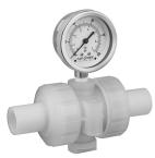
Unique in-line design eliminates "dead leg' that can harbor bacterial growth and contamination. Unpigmented thermoplastic material; FKM or metal ion-free EPDM. Special flexible elastomer spool separates system liquid from gauge fill liquid and assures accurate reading. Adaptable to existing piping systems. Sizes: 1/2" to 2".
